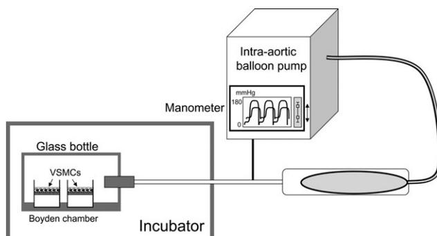
**Figure 1** Schema of the original apparatus with a Boyden chamber. This apparatus enables us to generate variable types and magnitudes of pulsatile pressure that are loaded on vascular smooth muscle cells.
